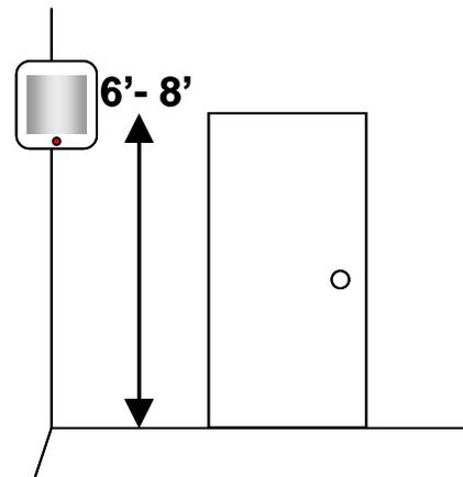
To mount EZMotion+ to the wall, separate the two halves of the enclosure by pulling gently downwards on the tab on the bottom. The back half of the enclosure can be attached to the wall using double-stick tape or by screwing it into the wall. Screws are recommended. Drill a 1/8" hole thru the EZMotion+ enclosure and the wall and mount with a drywall screw. Drill thru one of the screw locations in the back of the enclosure to ensure the screw will not interfere with the battery pack.
