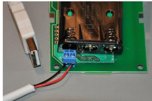
Note: The original EZMotion Rev 1.x did not have the blue power block. The wires must be connected to the battery holder connector directly. The Black wires goes on the center spring holder near the LED. The red wire goes on the + connector next to the LED as shown here.
